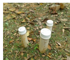
Figure 14. PVC pipes with activated charcoal filters inside, placed in the soil at IPEN.
