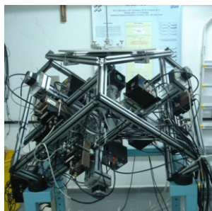
Figure 4. PAC spectrometer set up with six \text{BaF}_2 detectors.
